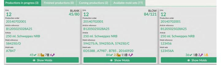
By consulting SIL, the operator will see at a glance how many moulds are available, how many are in repair or how many are scrapped.
